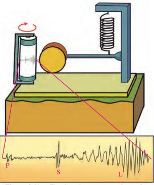
Figure 2.11 : Simple seismogram and graph
