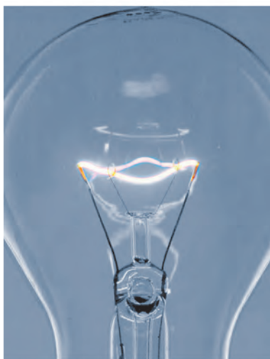
Fig. 14.12 Glowing filament of an electric bulb (incandescent)
