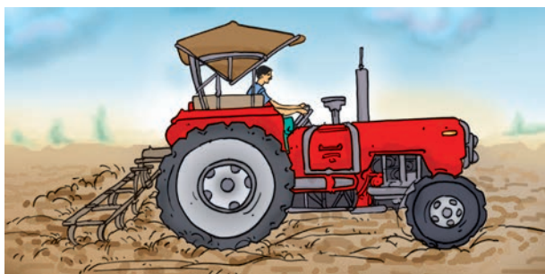
Fig. 1.1 (c) : Cultivator driven by a tractor
