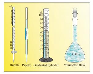
Fig. 1.7 Some volume measuring devices
